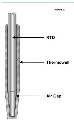
The following test program is designed to help nuclear power plants with Resistance Temperature Detector (RTD) performance verification. These tests shall be performed on new RTDs and/or new thermowells, or each time an RTD is removed and reinstalled in its thermowell. Also, the tests shall be performed after each period of extended outages (twelve months or more), especially if there is any reason to believe that the RTDs might have been disturbed during the outage.
