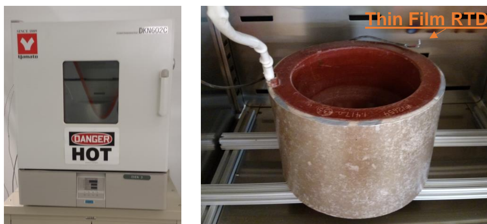
Figure 2. CRDM Lift Coil in Oven with Thin Film RTD
