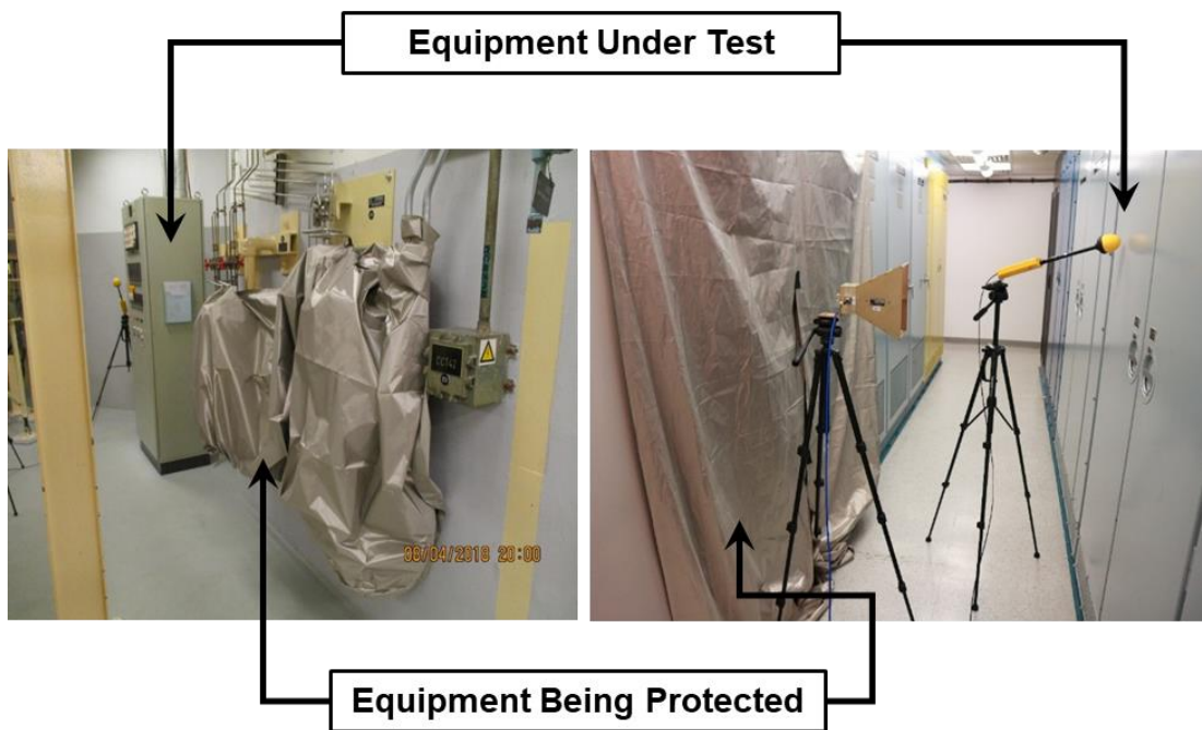
Figure 4. In-Situ Immunity Testing in a Nuclear Power Plant with Nearby Equipment Protected through Lightweight EMI Shielding Fabric
