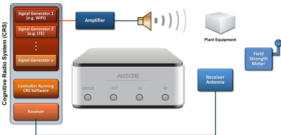
Figure 3. Block Diagram of AMS Cognitive Radio System (CRS Tool)
