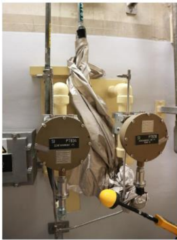
Figure 6. Example of Equipment Modifications Made to Mitigate Vulnerabilities Identified During In-Situ Wireless Immunity Testing (Note Temporary Shielding Material in Picture)
