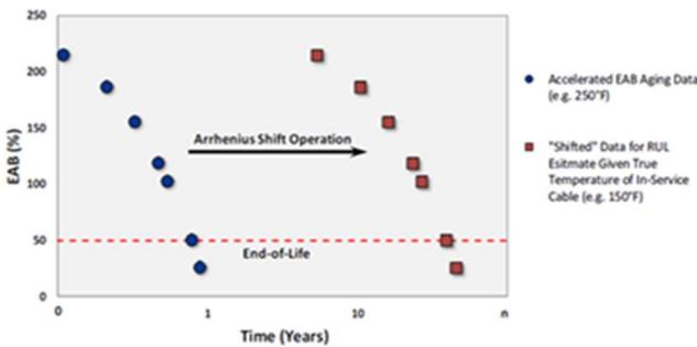
Fig. 2. Example of RUL Estimation Using Accelerated Aging EAB Data
