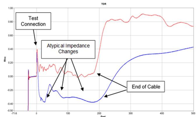
Fig. 4. Example Reflectometry Data Acquired for Originally Installed (Blue Trace) Cables and New Cables (Red Trace)
