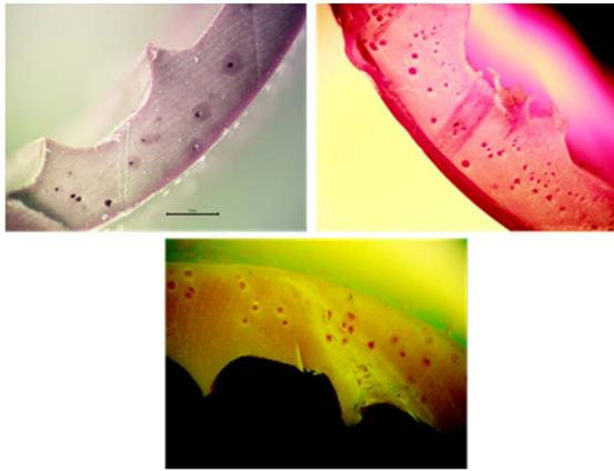
Fig. 5. Microscope Images Acquired at 20X Magnification showing Examples of Micro-voids in PVC Insulation of Originally Installed Cables
