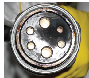
CRDM Connector Following Pin-to-Pin Short
