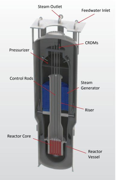
This model, which is based on the NuScale Power, LLC design, was produced using 3D printing technology to better visualize the unique geometries associated with SMRs.
