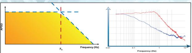
Figure 1. Illustration of Frequency Response of a First Order System and Actual Nuclear Plant PSDs
