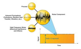
Figure 2. Illustration of Noise on the Output of a Pressure Transmitter
