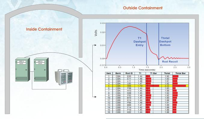
AMS provides automated test equipment for quickly performing rod drop time measurements in Westinghouse Pressurized Water Reactors (PWRs) in just minutes. Rod drop time testing is performed in PWRs to measure the time required for control and shutdown rods to travel from the fully withdrawn to the fully inserted position. The test allows for Digital Rod Position Indication (DRPI) power to remain on by using the AMS Patented Power-On Rod Drop Time Measurement technique.
